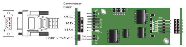
IMPORTANT! Make sure the power jumpers are set properly for 5 VDC regulated or 7.5 - 24 VDC unregulated power before supplying power to the board.
