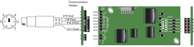
IMPORTANT! Make sure the power jumpers are set for Power from Port. WARNING! DO NOT CONNECT POWER TO THE POWER HEADERS!!
