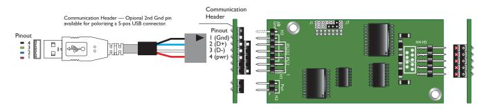
**NOTE:** Make sure that you have set the jumpers for power-from-port before connecting to the USB port.
